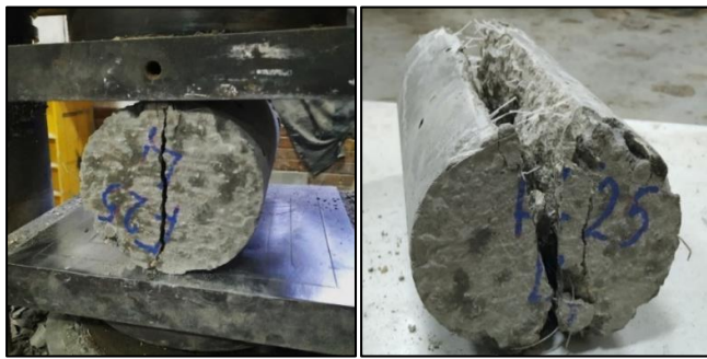
Fig. 12: Failure section for cylinders with polypropylene fibers
