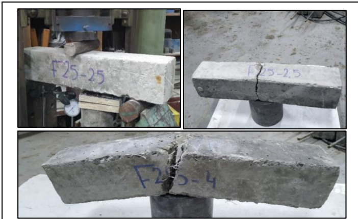
Fig. 16. Failure section for prisms with polypropylene fibers prisms
