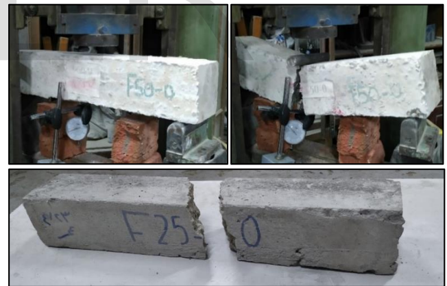
Fig. 15: Failure section for control prisms without polypropylene fibers
